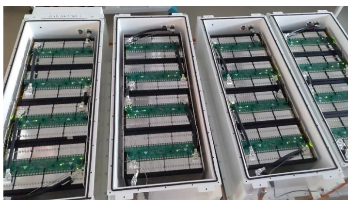
Figure 10 – Open-top picture of the battery during factory test at Bluways (ORCA) [8]
