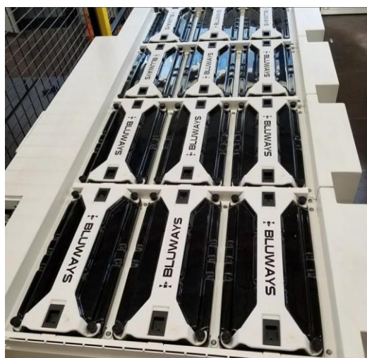
Figure 11 – Top picture of the LiC during power split testing at VUB (ORCA) [8]
